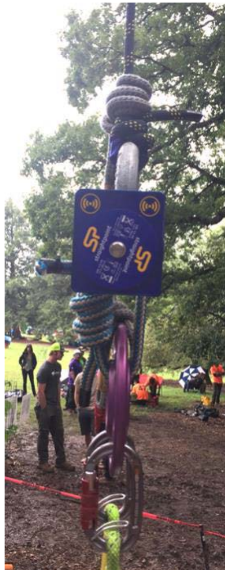
Figure 1 shows the Straightpoint LLC load cell used to measure forces during the Ascent event at the 2017 ITCC in Washington, DC.
